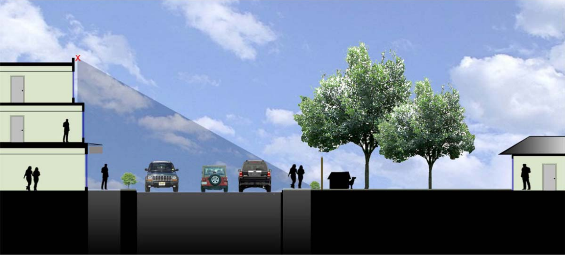
Bendel Street Section - Proximity Slope 33 degrees
